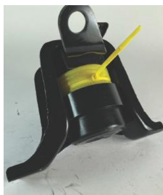
Figure 5: Feed cable tie around Ring with head on outside
