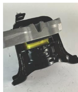
Figure 6: Tighten cable tie to close the gap
