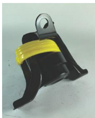
Figure 1: 'Hook' one end of the ring over the outside of the bracket to assist fitting
