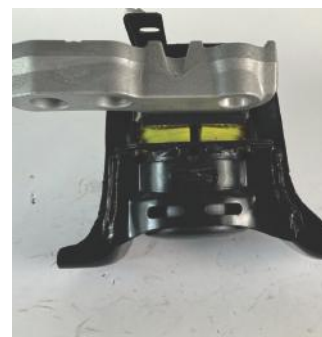
Figure 4: Line the split line up underneath the post
