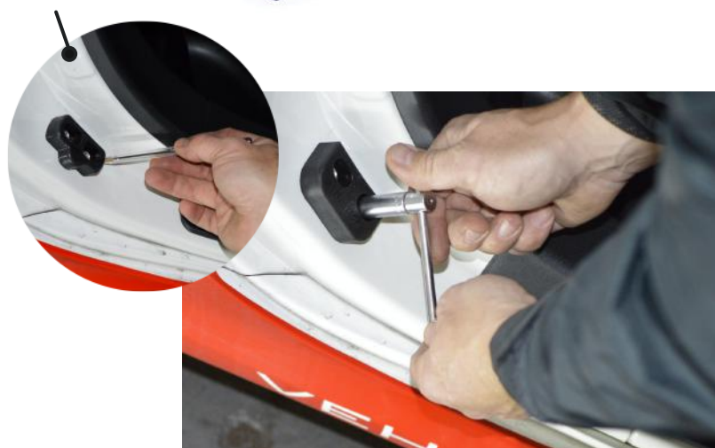
Figure 1 - how to position the polyurethane bush
