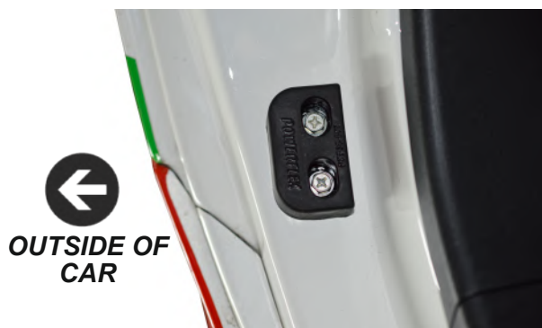
Figure 1 - how to position the polyurethane bush
